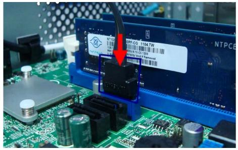
6. Let HDD SATA data cable pass through the two metal clip.
